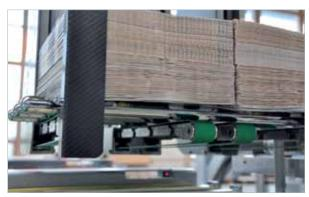
Bundle transfer to the Servo-double-gripper
