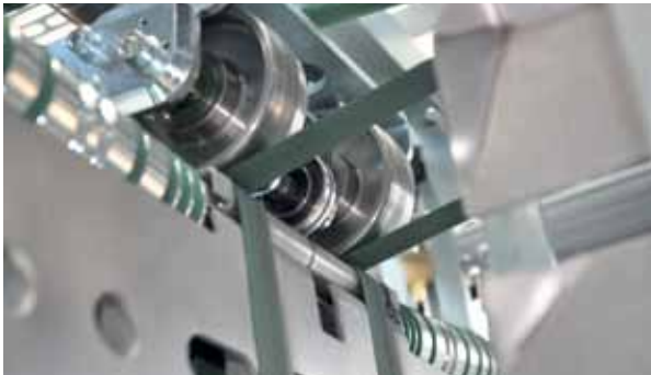
Stabilization of the shingled stream by round belts and a special finger-type
